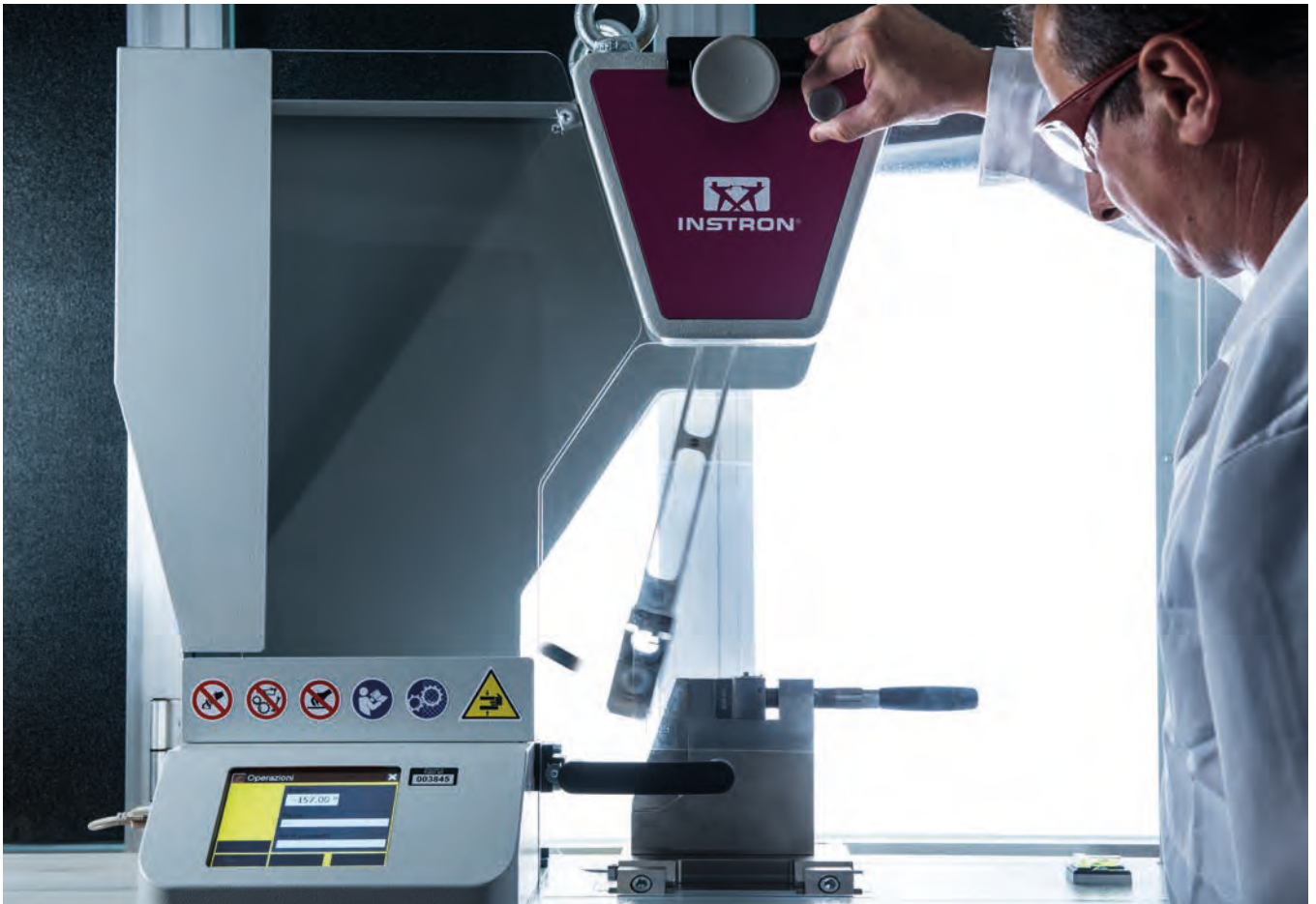
Impact test with pendulum.
